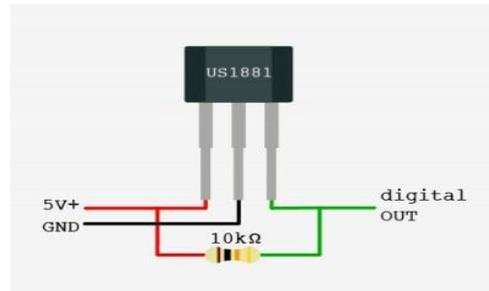
Figure 8.3.2 The pinout diagram for a Hall effect sensor
