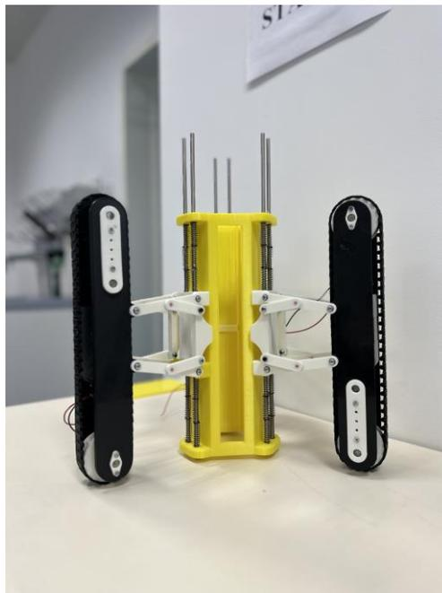
Figure 8.4.1 The assembled In-pipe robot v1.0.
