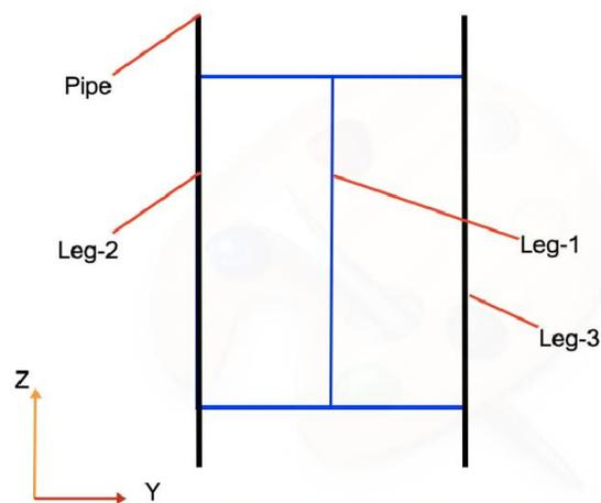
Figure 9.1.2 – Junction between the crawler modules and pipe wall
