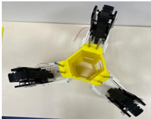
Figure 8.4.2 Top view In-pipe Robot v1.0
