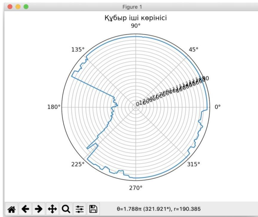
Figure 1.4 – Visualization of pipe's internal structure.
