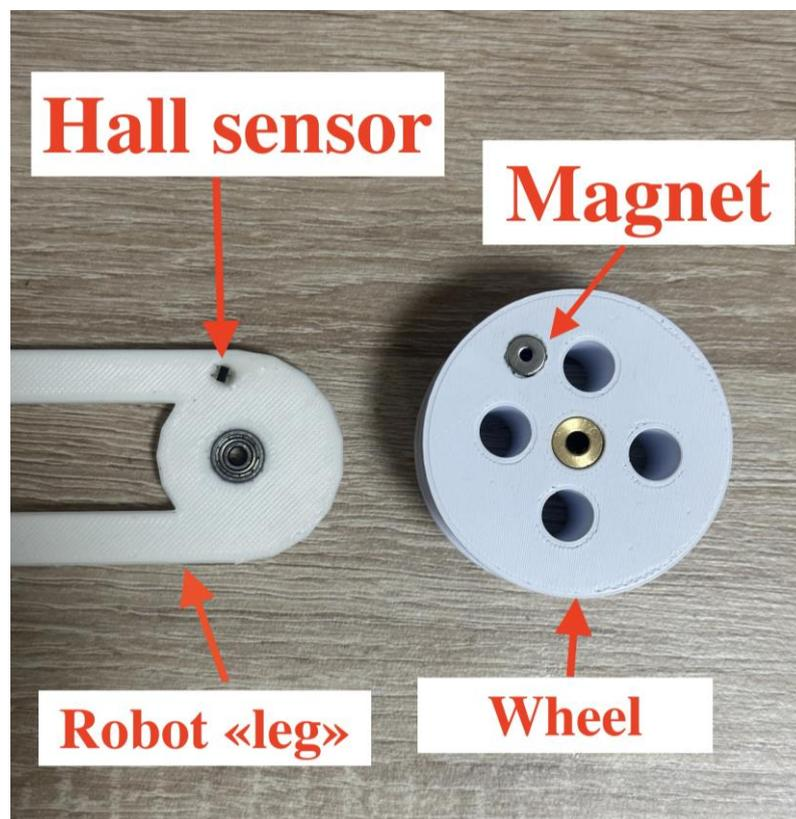
Figure 8.3.3 – Installing the sensor and magnet
