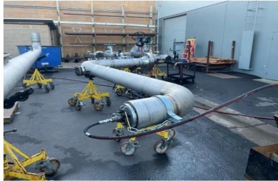
Figure 5.4 – Pipe Pressure Testing
