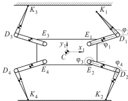
Figure 7.3 – Diagram of the in-pipe walking robot.
