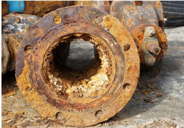
Figure 1.2 – Presence of debris and rust in pipe
