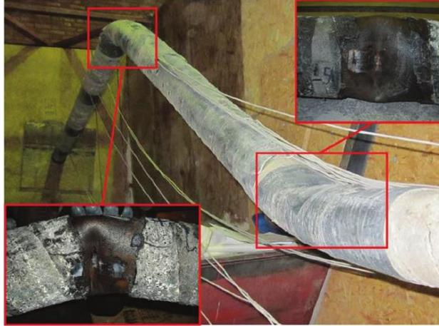
Figure 4.4 – Pipe deformation
