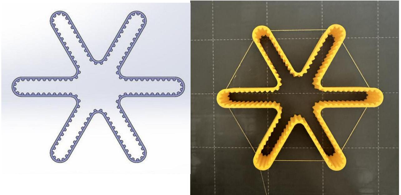
Figure 8.4– 3D and printed versions of belt
