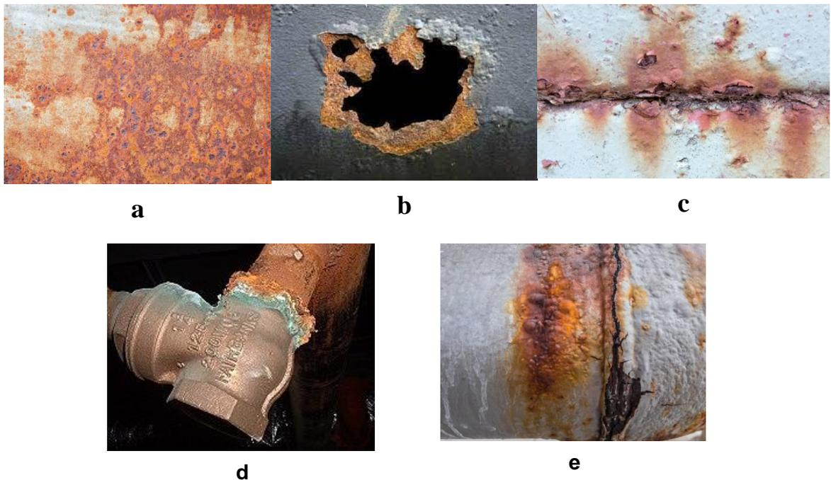
Figure 4.1 – Uniform(1), Pitting(2), Crevice(3), Galvanic(4), Stress(5) corrosions.
