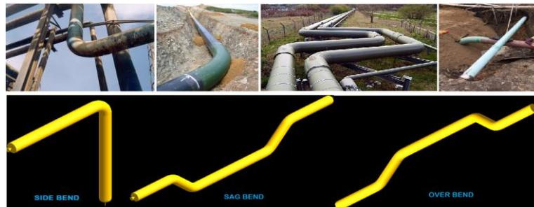
Figure 1.1 - Different types of bends in the pipeline.
