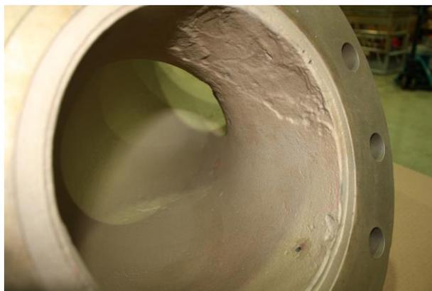
Figure 4.3 – Abrasion of inner wall of pipe
