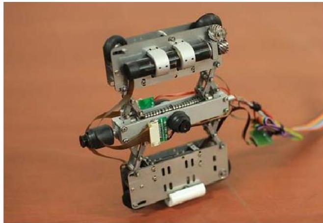
Figure 7.1 – Wheel driven robot
