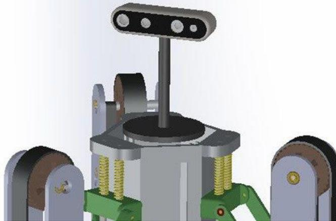
Figure 6.1.1 – TOF sensor mounted on the robot
