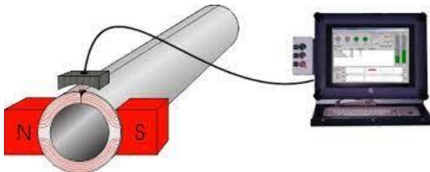
Figure 5.3 – Magnetic Flux Leakage
