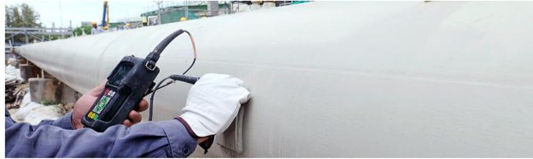
Figure 5.2 – Ultrasonic testing
